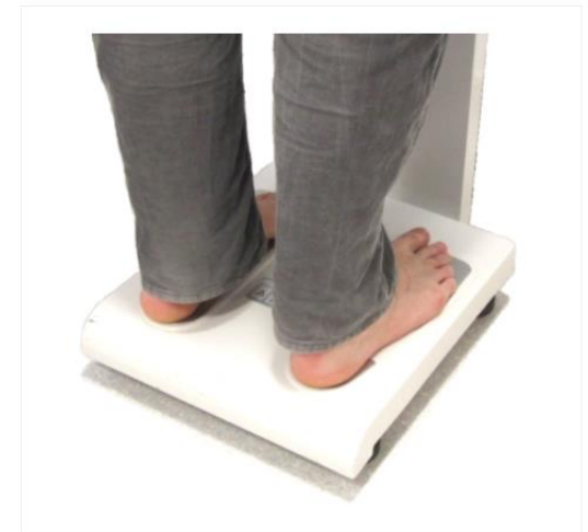
Figure 2 Participant's feet touching the electrodes on a foot to foot body composition monitor. Source: MRC Epidemiology Unit.
